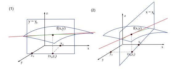
**Figure 6:** Geometrical picture of  $\partial f/\partial x$  (1) and  $\partial f/\partial y$  (2) at the point  $(x_0, y_0)$ . In (1)  $\partial f/\partial x$  is the slope of the red line which is tangent to the green curve resulting from the intersection of f(x, y) and the plane  $y = y_0$ . In (2)  $\partial f/\partial y$  can be identified in a similar fashion.
