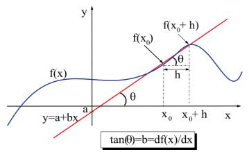
**Figure 5:** Geometrical picture of df/dx at the point  $x = x_0$ . Applying the definition (2.47), the derivative is nothing but the slope of the line y = a + bx which is tangent to f(x) at the point  $x_0$ , namely  $b = \frac{df}{dx}|_{x_0}$ .
