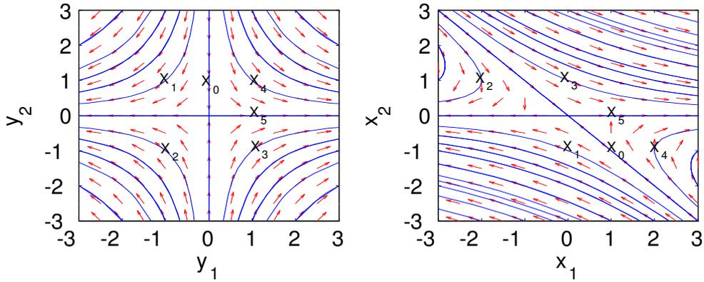
**Figure 5:** Phase portraits for the linear systems  $\dot{y} = Jy$  and  $\dot{x} = Ax$ .
