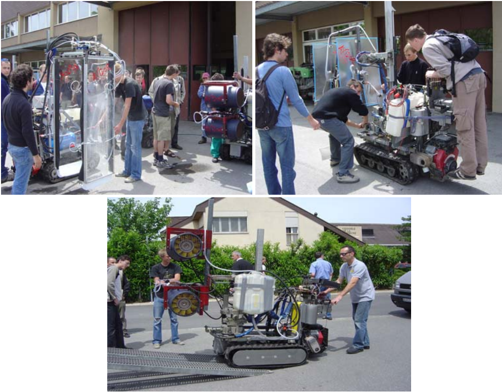
Figure 4 Preparation of spraying equipment for field test
