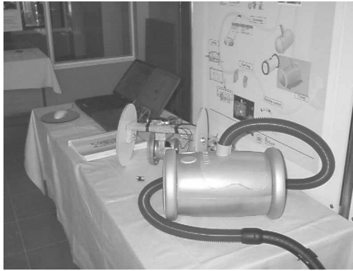
Figure 6. The prototype of a vacuum cleaner (front) and one of the mock-ups (back).
