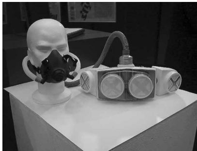
Figure 7. The prototype of a respiratory unit for welders.
