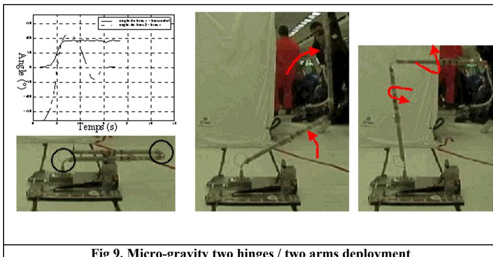
Fig 9. Micro-gravity two hinges / two arms deployment
