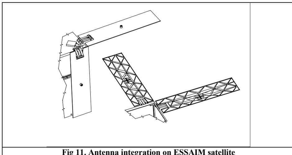
**Fig 11. Antenna integration on ESSAIM satellite**
