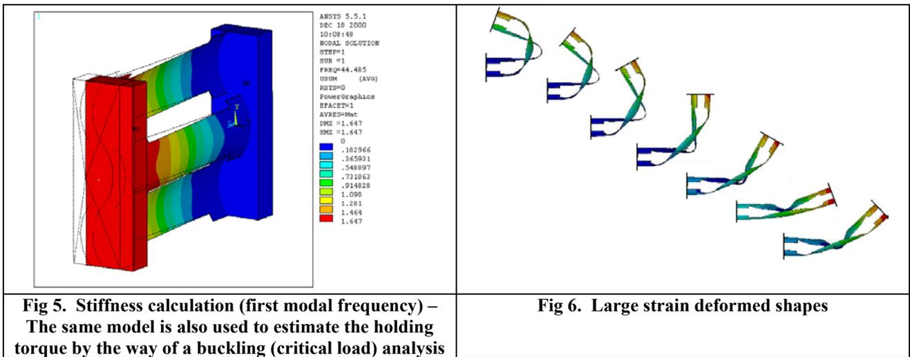
A buckling calculation (critical load) leads to define the holding torque, namely the effort the hinge can stand, under satellite attitude control, without unlocking. This latter is performed on the same numerical model as the previous one (see Fig. 5).
