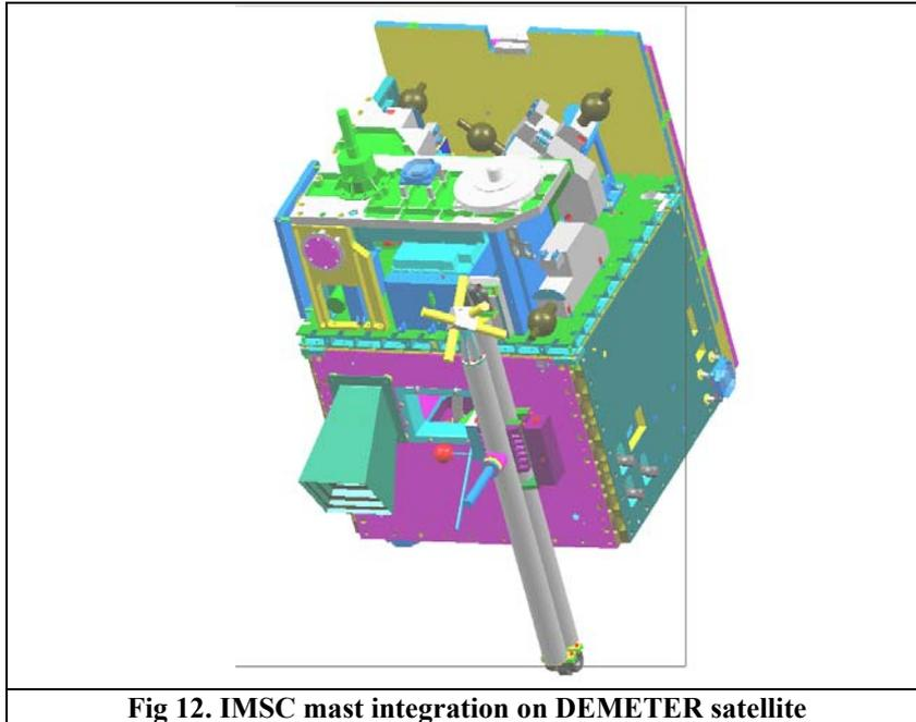
**Fig 12. IMSC mast integration on DEMETER satellite**
