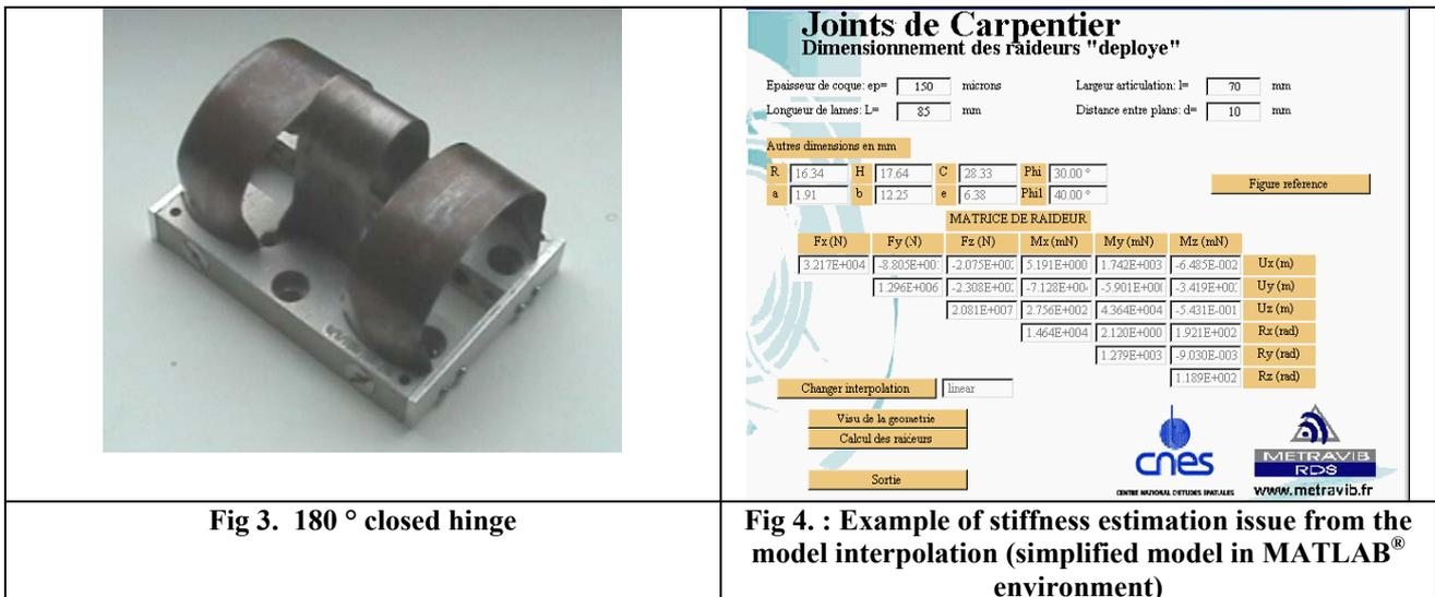
Fig 3. 180° closed hinge
