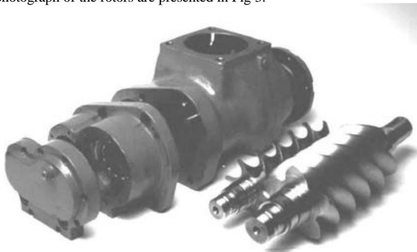
**Fig. 2 Oil injected screw compressor with 'N' rotors.**
