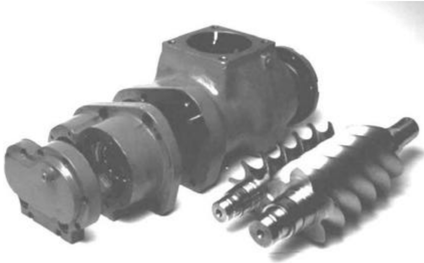
Figure 3 Oil injected screw compressor with 'N' rotors.
