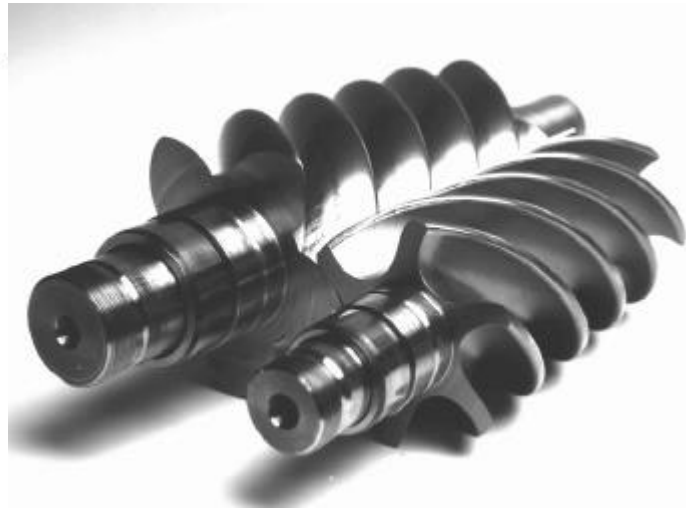
Figure 4 Drawing and photograph of 5/6 male and female 'N' rotors
