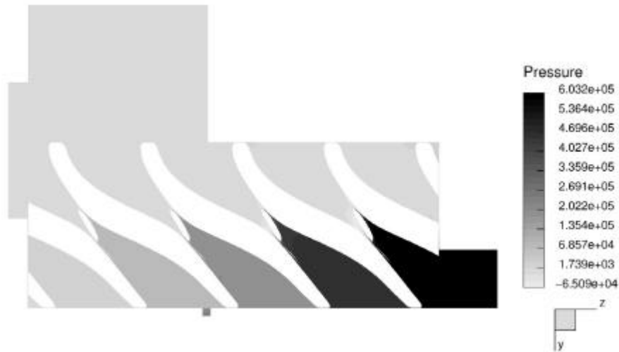
Figure 6 Pressure field in the axial cross section between rotors
