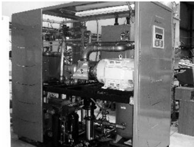
Fig 9 ORC Demonstration Unit
