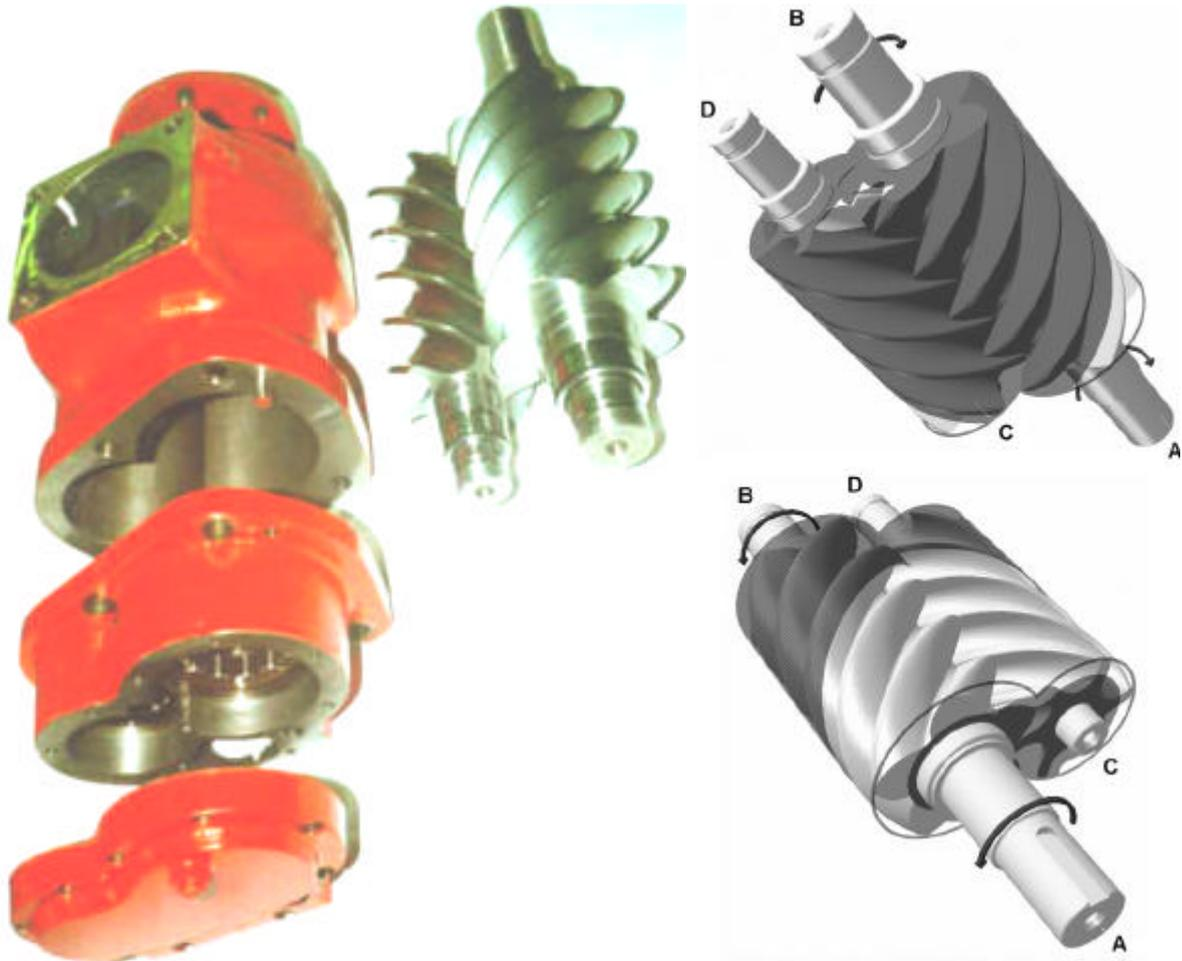
**Fig. 1 Screw compressor principal mechanical parts**
