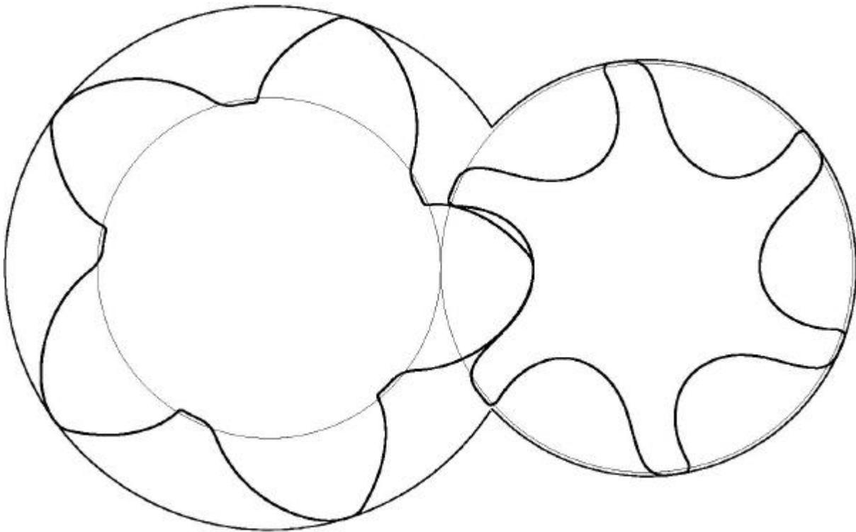
**Fig. 5 Rotor profile optimized for a refrigeration compressor duty**
