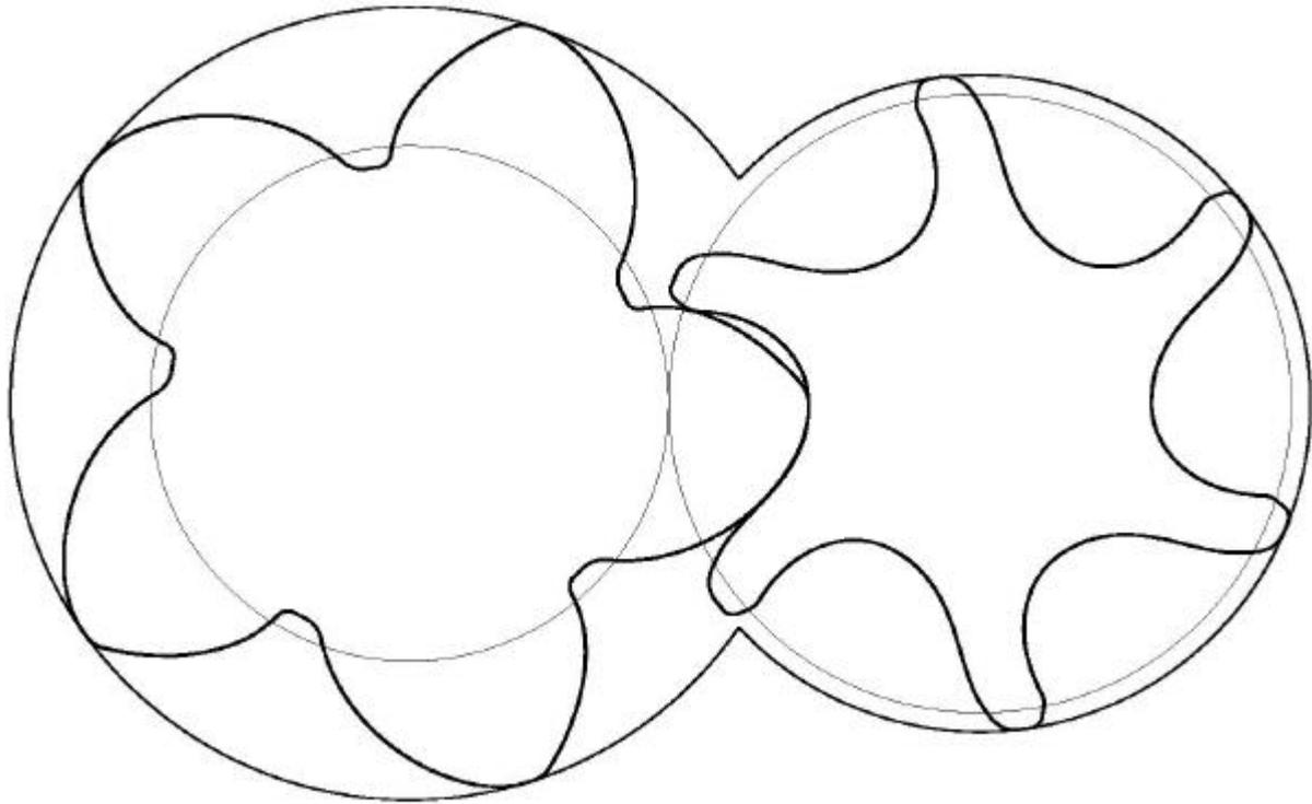
**Fig. 3 Rotor profile optimized for an oil-free air compressor duty**
