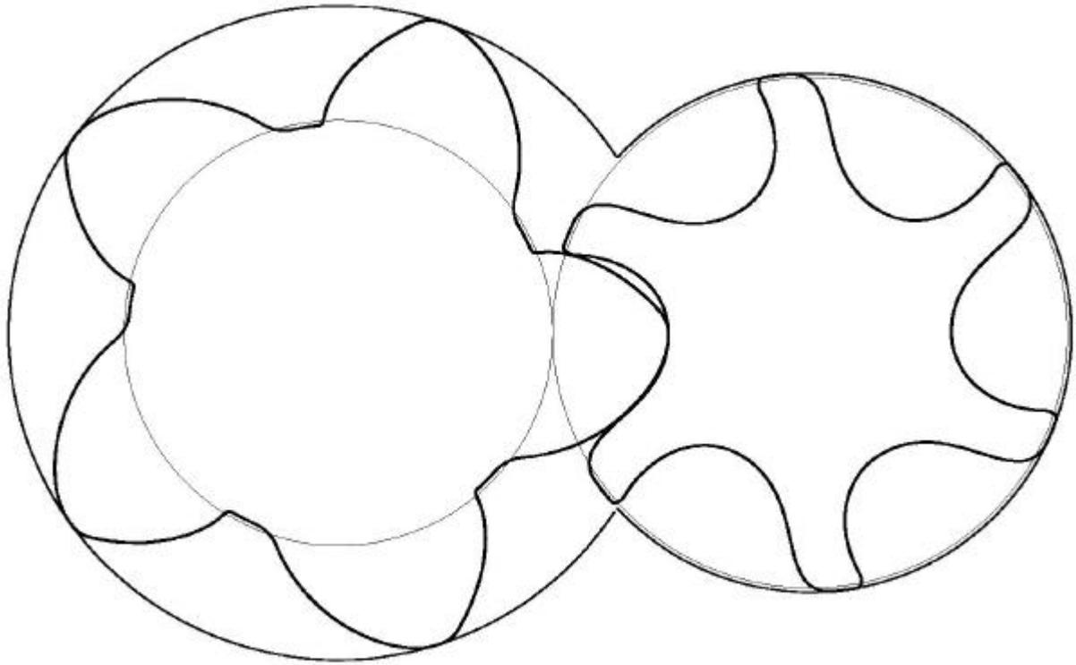
**Fig. 4 Rotor profile optimized for an oil-flooded air compressor**
