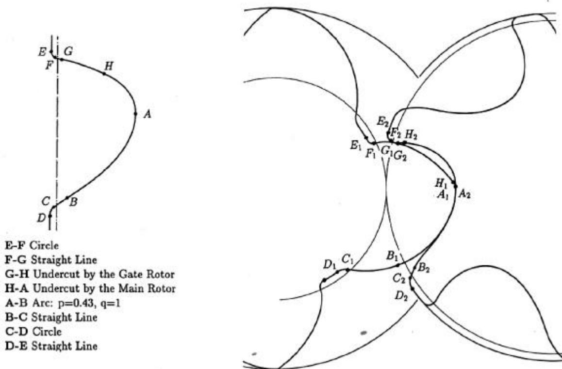
**Fig 2. Distribution of generating profile curves on the rack for 'N' rotors**
