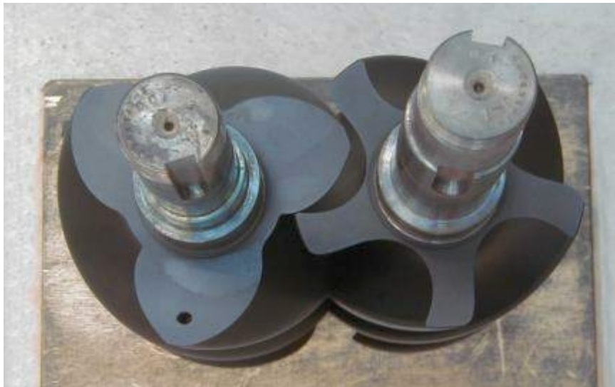
Fig. 12 3/5 Rotor profile optimised for an oil-free compressor
