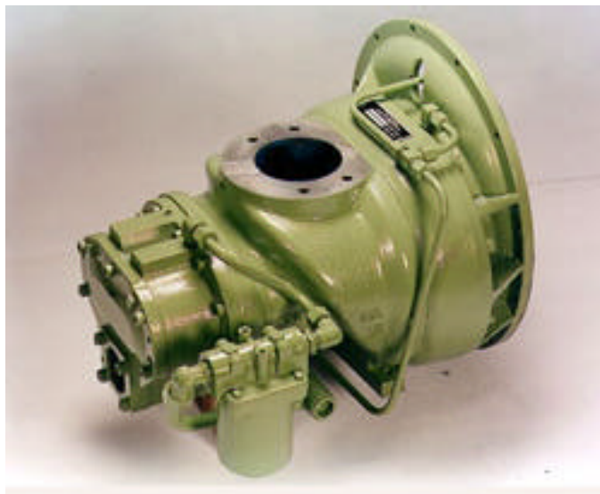
Fig.4 Compressor with Replacement Rotors installed
