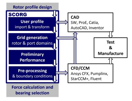
SCORG<sup>™</sup> offers unique capability for performance evaluation of screw compressors, pumps and motors by use of Computational Fluid Dynamics and Thermodynamic Multi Chamber Modelling.
