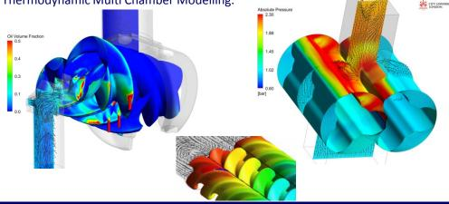
SCORG directly links grid and case setup with CFD Solvers:
