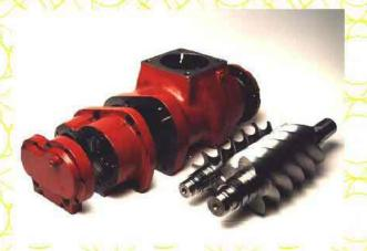
"N" rotor profiles for screw compressors, based on a patented rack generation procedure, offer greater flow area, less leakage, smaller internal friction and greater tooth strength than any other known rotor profile. Starting with these, or any other rotor profile types, the Centre can perform accurate performance predictions followed by complete detail design of compressors for any application.
