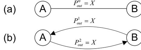
**Fig. 1.** (a) Undirected link (b) Transformation to two anti parallel directed links
