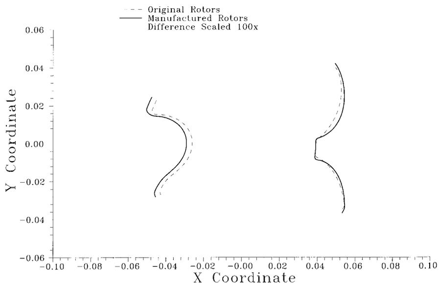
Fig. 7 Rotor profiles generated from a given tool
