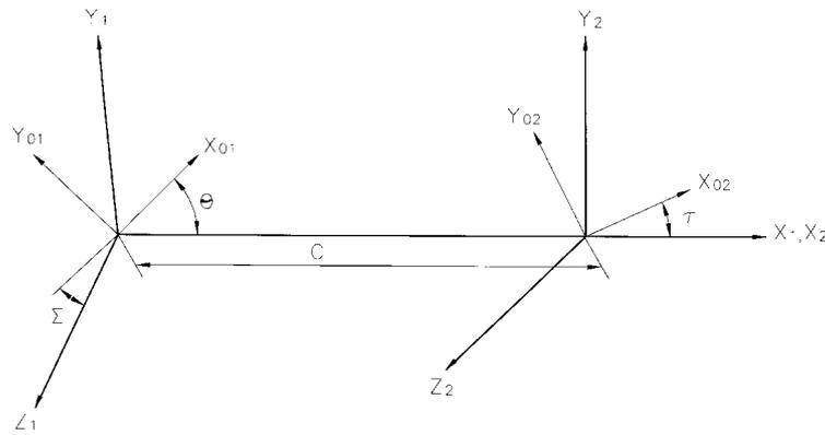
Fig. 2 Coordinate systems of crossed helical gears
