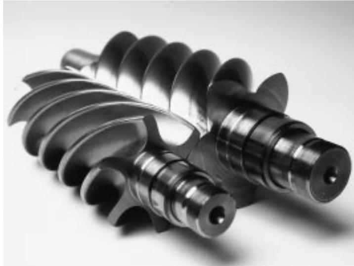
Fig. 1 Screw rotors in mesh
