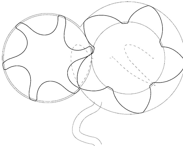
Fig. 4 'N' rotors in mesh, sealing line and clearance distribution
