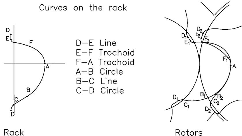
Fig. 3 'N' rack and rotor profile points
