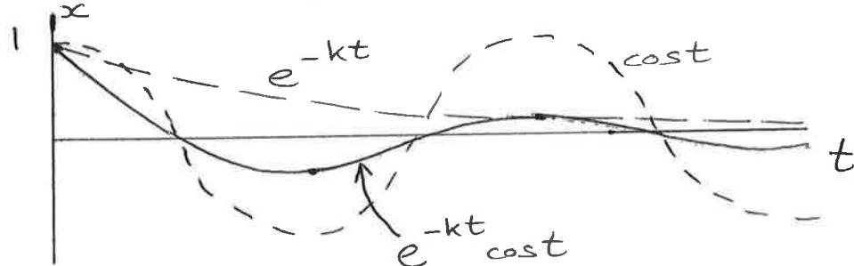
The oscillation is said to be modulated in amplitude by  $e^{-kt}$
