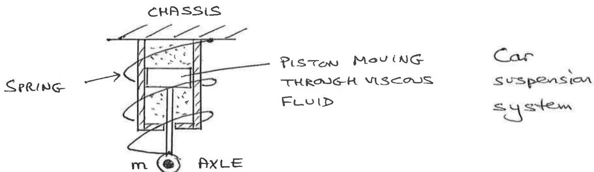
Typically suspension system is damped by the movement of a piston through hydraulic fluid, to avoid too much 'bounce'.
