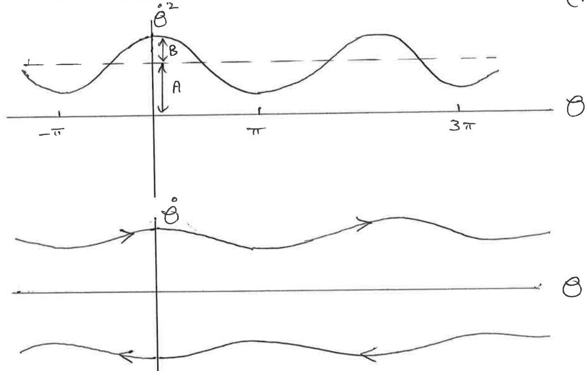
The pendulum completes whole circuits in either the clockwise or anti-clockwise directions.
