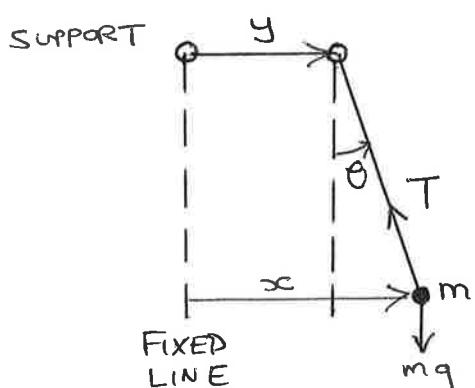
Support moves with displacement  $y(t)$ . Tension  $T$ .
