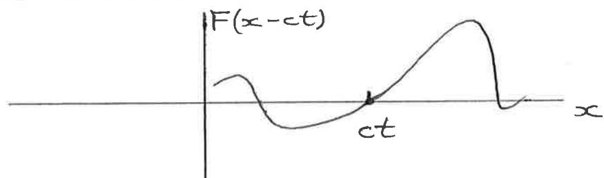
i.e. it represents a wave travelling in the +ve  $x$  direction with speed  $c$ .
