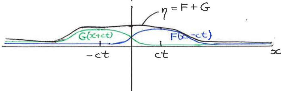
Waves propagate in each direction with speed  $c$
