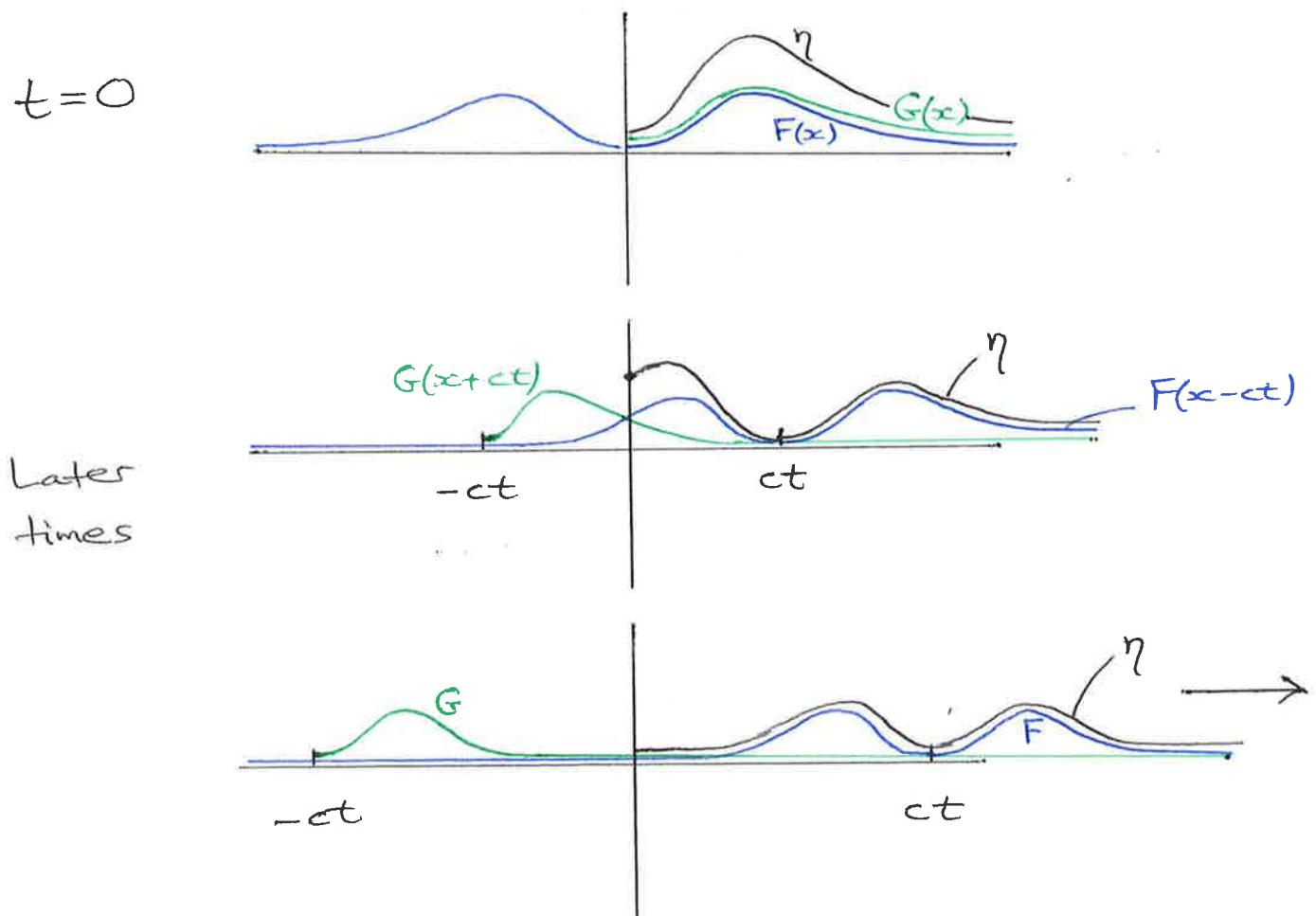
The inward travelling component is reflected, producing a 'double' profile travelling outwards.
