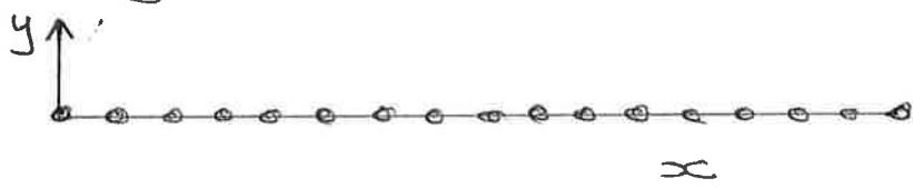
We allow the string to move in the transverse direction and denote the displacement by  $\eta(x, t)$ .
