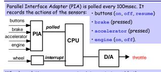
Wheel revolution sensor generates interrupts to enable the car speed to be calculated.
