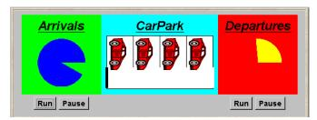
A controller is required for a carpark, which only permits cars to arrive when the carpark is not full and does not permit cars to depart when there are no cars in the carpark. Car arrival and departure are simulated by separate threads.
