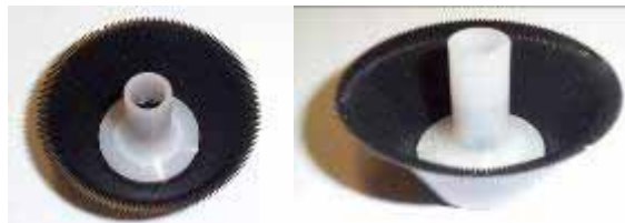
Figure 6: the striated cup of the prototype
