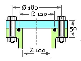
The cover of a pressurised cylinder is attached by a self-energising seal and 6 identical bolts M10x1.5 of class 8.8. The fluid pressure is essentially constant at 6 MPa. A safety factor of three is required. Check if the given bolt can sustain the pressure!
