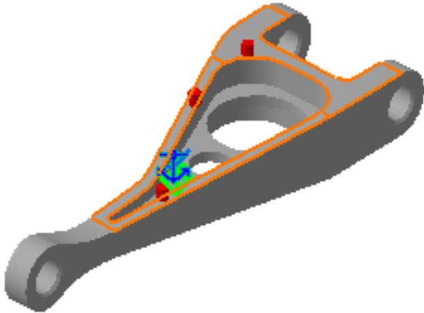
4. Enter a new Mass Density in the Surface Mass Density dialog box. In this particular case, enter 50kg\_m2.
