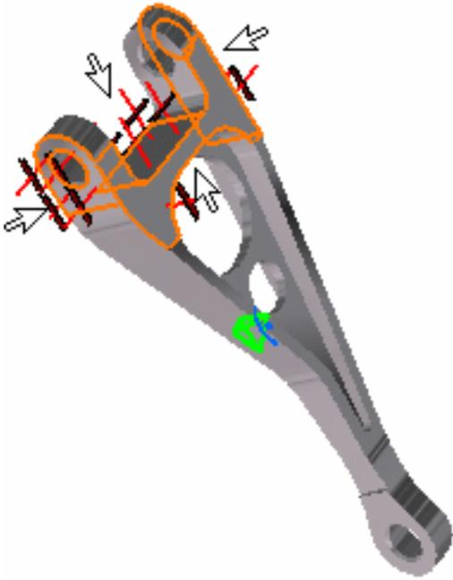
Symbols representing the surface sliders appear as you select the four faces. The elements supporting the surface slider are automatically displayed in the Surface Slider dialog box.
