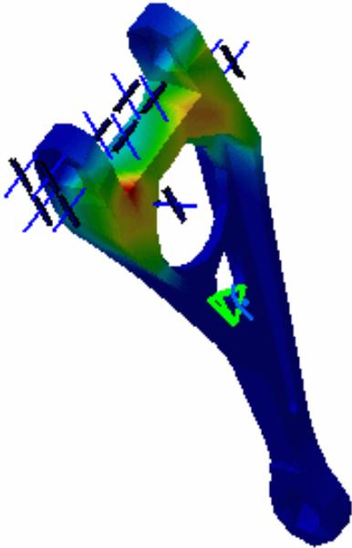
Both a Translational displacement vector image object and a Von Mises Stress (nodal value) image object appear in the specification tree under the Static Case Solution.1 objects set.
