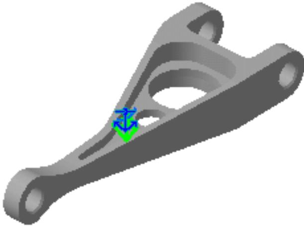
The Iso-static Restraint object (`Isostatic.1`) has been inserted under the `Restraints.1` objects set in the specification tree.
