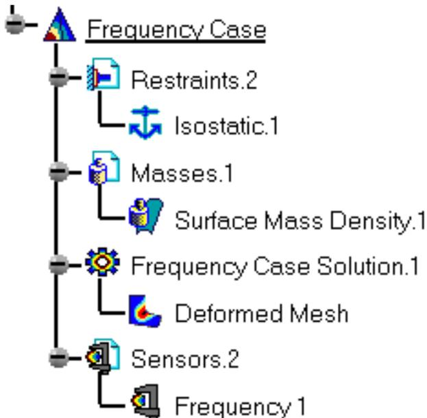
2. Double-click the `Deformed Mesh` object in the specification tree to edit the image.
