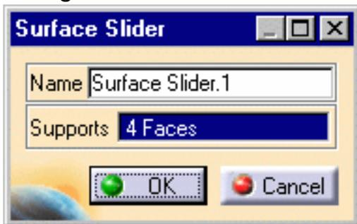
4. Click OK in the Surface Slider dialog box to actually create this surface slider.
