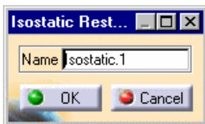
You will restrain your part in such a way that it is statically definite and all rigid-body motion is impossible. The program will automatically determine the restrained points and directions.
