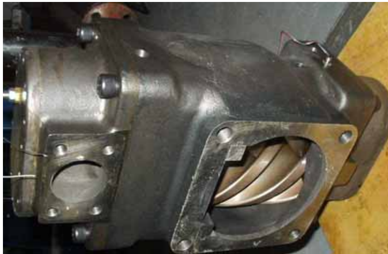
Figure 8 Expanded View of the Compressor-Expander for Fuel Cell Application
