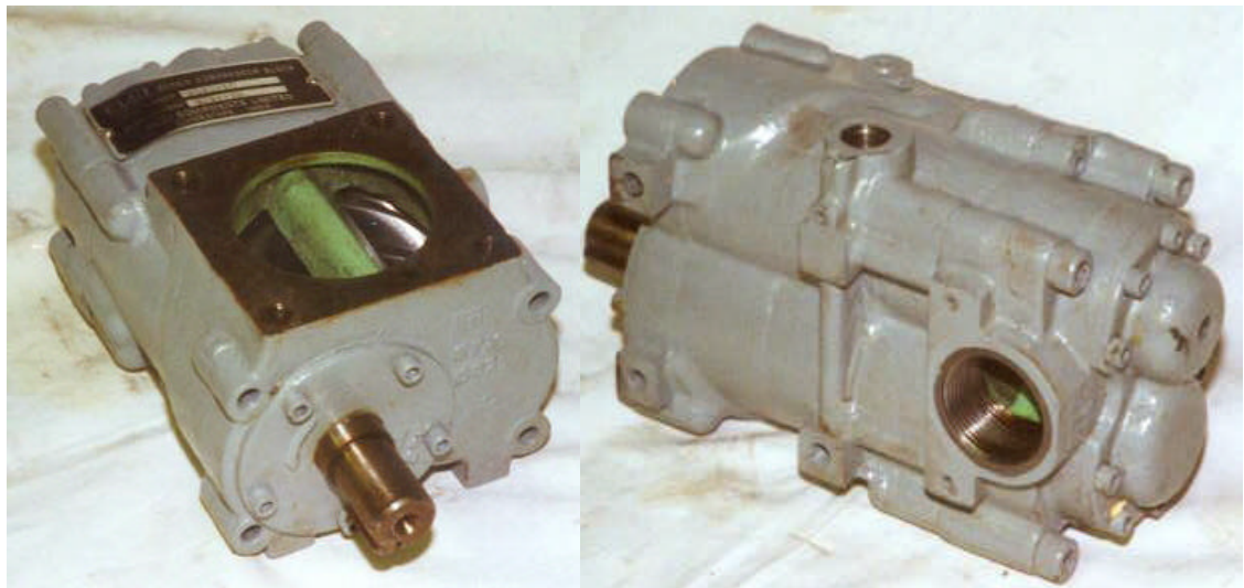
Fig. 3 The smallest compressor of the family, 4/5-73 mm
