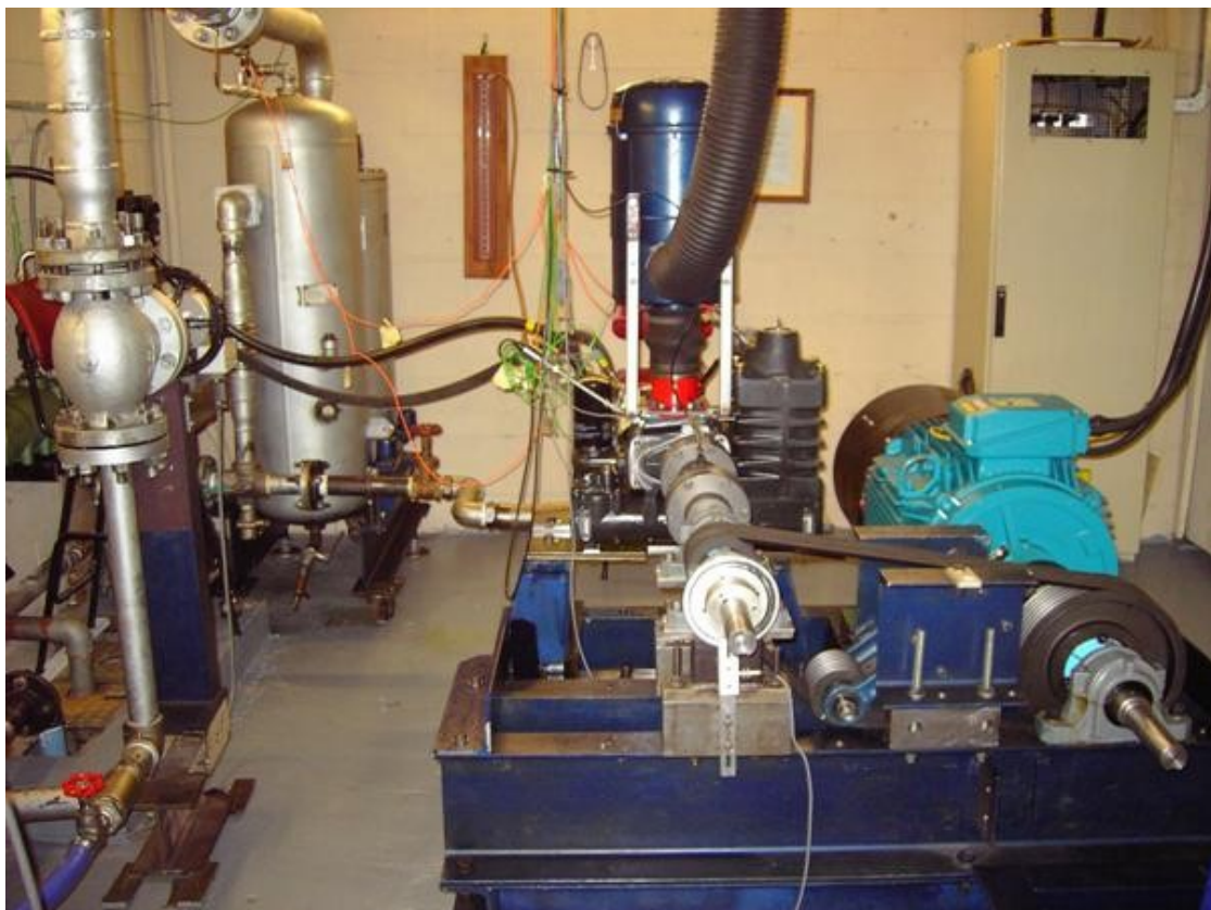
Fig 5. Screw compressor in the test rig
